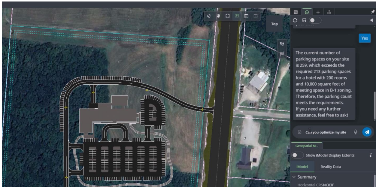
Bentley's OpenSite+ software with copilot uses organization-specific documents and design models for quick insights and edits. (Photo Bentley Systems)
